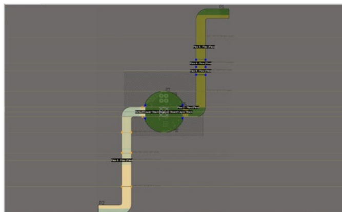
Figure 9: Board regions are assigned the required layer stacks for rigid and flexible areas to be defined, and bending lines are added.
