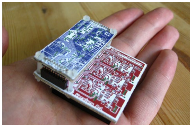
Figure 3: PCB paper doll using cardboard, mounting posts and connectors [2] .
